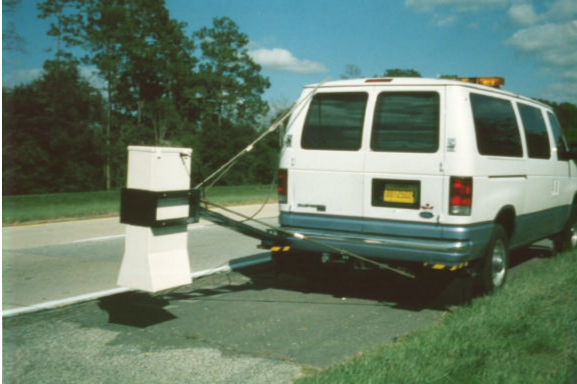
Figure 1 Photographic Illustration of FDOT GPR van
