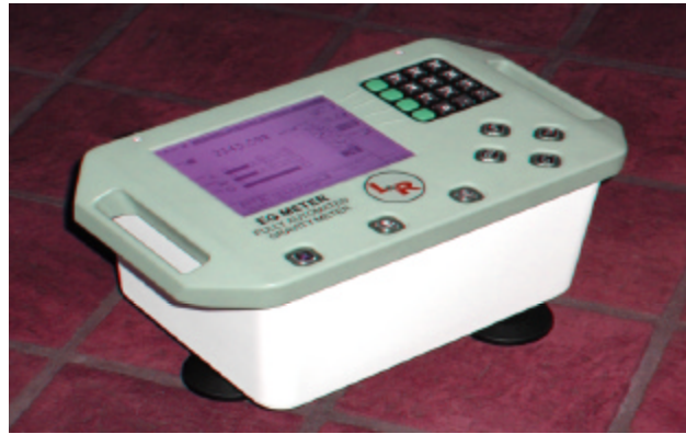
Figure 1. A Lacoste and Romberg model E gravity meter that can be used for all types of gravity surveys. Adapted from Lacoste and Romberg Inc.
