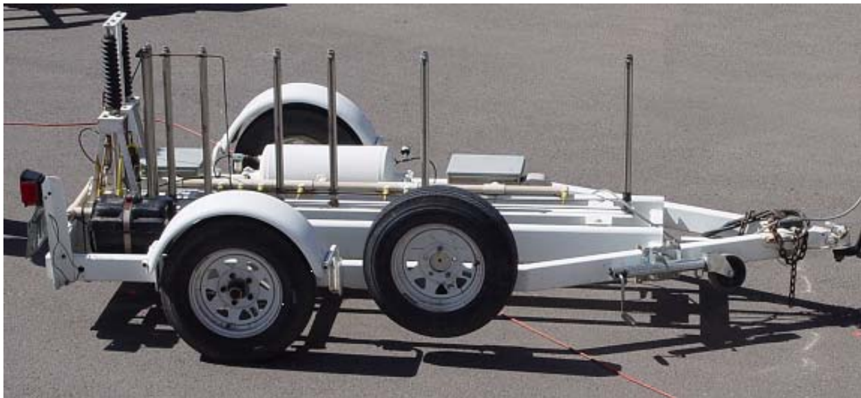
Figure 2 - Seismic Pavement Analyzer (SPA)
