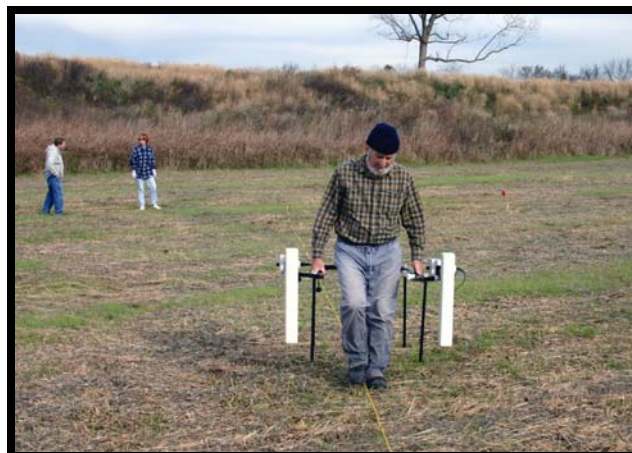
Figure 4. Duplexed Geoscan Research Fluxgate Gradiometers Used in These Surveys.
