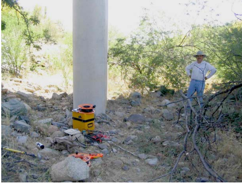
Figure 6. Starting location of the seismic line adjacent to Pier 2. Results of this line are presented in Figure 7. Note very coarse particles in the streambed. A scan line using a 100-foot (30 m) cloth tape was performed at this location to provide a very coarse particle size distribution. D_{50} and D_{95} for the surface particles were 0.5 and 11.2 inches (12.5 and 284 mm), respectively. The largest particle counted had a b-axis dimension of 17.3 inches (440 mm).
