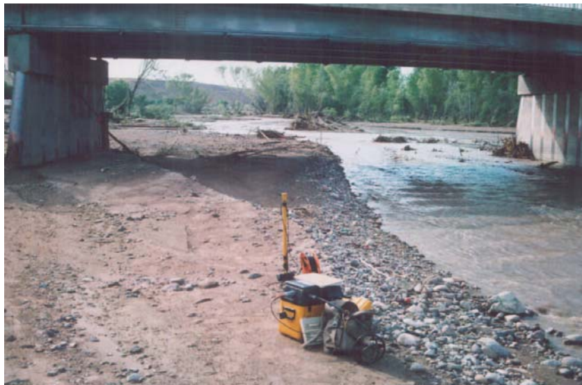
Figure 2. seismograph with 4.5 Hz geophone array deployed along active stream bank under bridge. P-wave data was collected using the sledgehammer energy source with the instrument set to 0.063 msec sample intervals and 256 msec sample period. S-wave data was collected using jogging alongside the array and traffic noise on the bridge with the instrument set to 1 msec sample intervals and a 12 second sample period.
