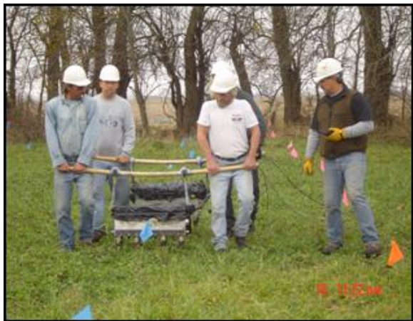
Figure 3: HRS acquisition using dual MicroVib source
