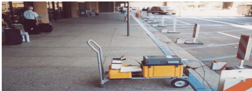
Figure 3: Vertical P-wave geophones were laid out along the curb to record noise for ReMi analysis. There was no need to close down the airport or disrupt normal operations during the survey, making ReMi attractive option in urban and congested areas.
